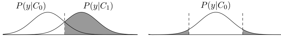
Figure 2.1: Absolute analysis and differential analysis, the two main approaches to fraud detection, are illustrated using a probabilistic view. In absolute analysis, illustrated left, models of both normal ( C_0 ) and fraudulent behavior ( C_1 ) must be formulated. In differential analysis, one model is built assuming normal behavior ( C_0 ) and any deviations from the established behavior are classified as fraudulent. The dashed lines indicate some arbitrary decision borders and the shaded area denotes the regions to be classified as fraudulent.
