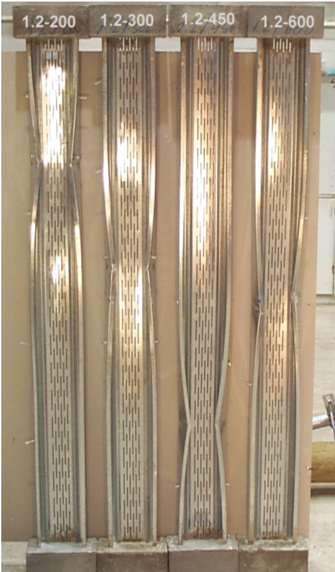
Fig C3: Failure modes of gypsum board braced web stiffened C-section short columns with thickness of 1.2 mm and length of 1800 mm.
