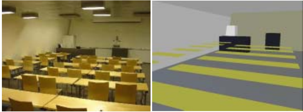
Figure 4.14: A photograph and the 3D model applied in auralization of the studied lecture room.
