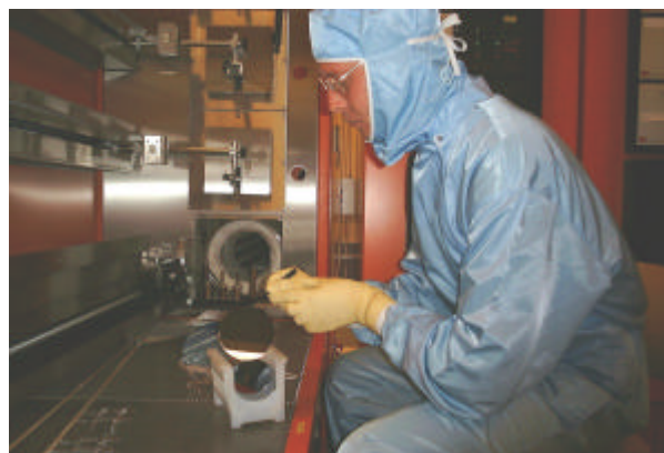
Figure 1.3. Processing: Jaakko Härkönen loading silicon wafers into an oxidation furnace at the MEC clean room.
