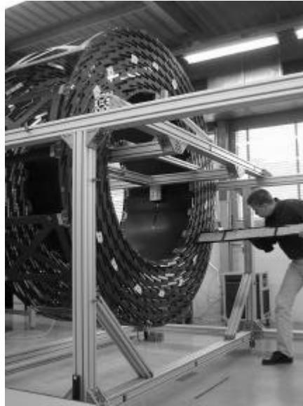
Figure 1.2. Tommi Vanhala inserting prototype support frames with silicon detectors in a prototype CMS Tracker Outer Barrel support wheel.
