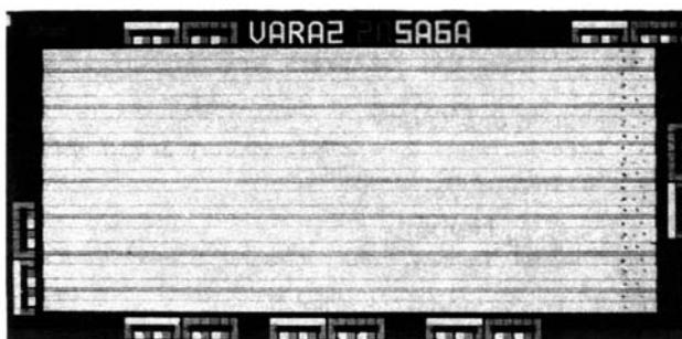
Figure 25. Micrograph of a stack containing 14 diodes.
