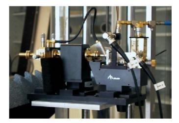
Figure 3.3 Photograph of the ABmm ESA-1 transmitter.
