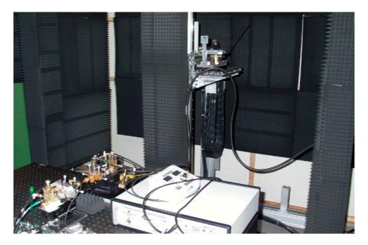
Figure 5.8. Test setup for verification of the phase correction accuracy. Scanner is at the center of the scanning area.
