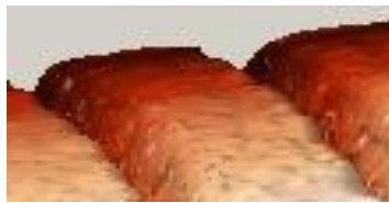
Figure 16: Surface morphologies based on AFM measurements of a-Si:H waveguides deposited by PECVD at 250^\circ\text{C} .
