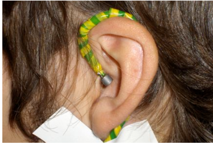
Figure 3.1: Microphone is inserted to the entrance of the ear canal.
