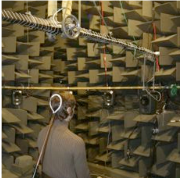
Figure 3.3: Measuring HRTFs. Loudspeaker at the end of the boom is the sound source.
