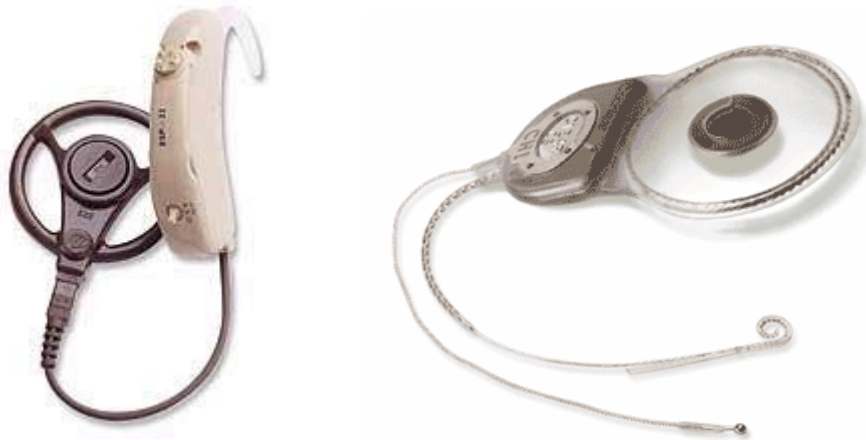
Figure 6. On the left the behind-the-ear microphone, implant processor and the transceiver (outer part). On the right the implanted part of the cochlear implant device (inner part). [64]
