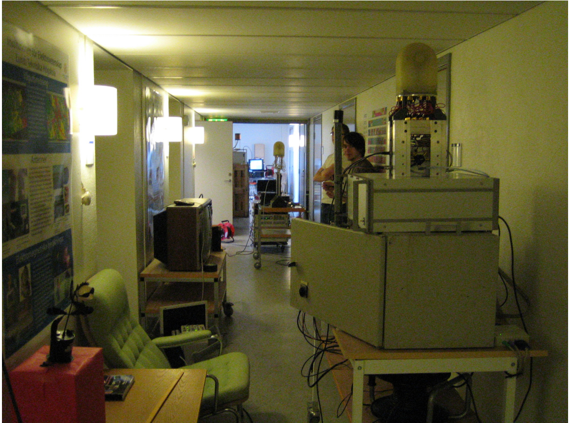
Figure 4.5: The measurement equipment in positions for a short range LOS measurement in the Radio Systems Laboratory corridor. The TKK RX is at the right in the front, The LU RX can be seen at the end of the corridor, and the LU TX is located in the middle of these two.
