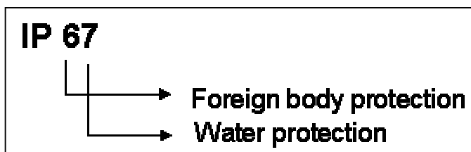
Figure 5. Example of IP marking
