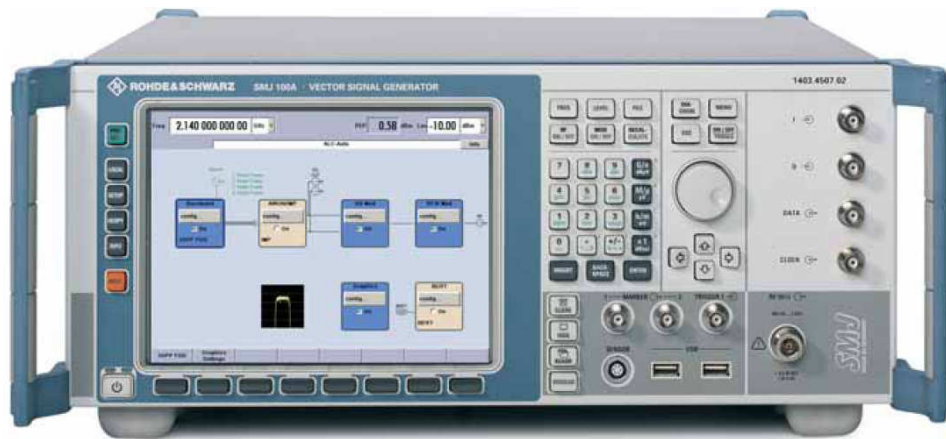
Figure 24: Rohde & Schwarz SMJ100A signal generator
