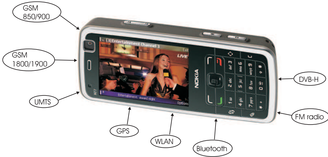
Figure 1.1: Nokia N77 and radio systems, which could be integrated into a mobile terminal. N77 includes only DVB-H(EU), GSM900, GSM1800/1900 and UMTS.
