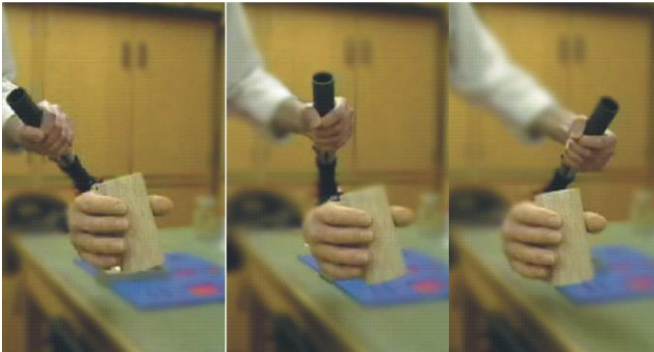
Fig. 8. Motion Compensation - The humeral section is rotated in a similar manner to humeral ab/adduction and the motion is detected by the accelerometers in the wrist and the wrist is driven to compensate for the motion.
