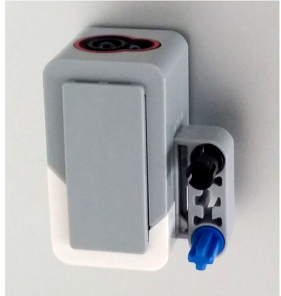
(b) Colour/light sensor (from EV3 platform used to detect reward related stimuli during the experiments.
