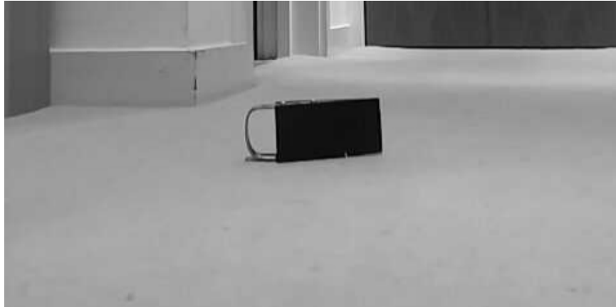
Figure 7.2: Unprocessed image from the camera frame-buffer with a resolution of 480 x 270 pixels and 8 bits colour depth..
