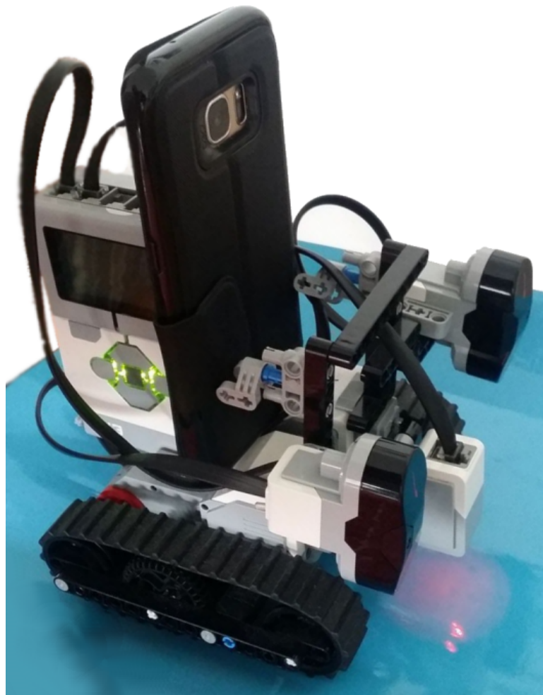
Figure 7.11: Experimental robot built with Lego-Mindstorms (EV3) and smartphone camera as visual system.
