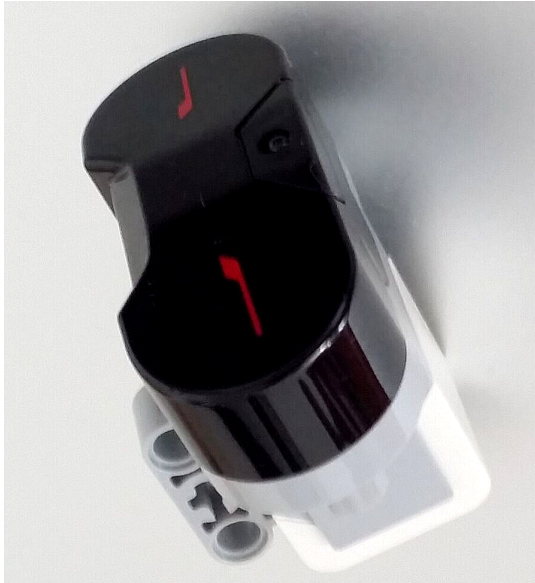
(a) Infrared sensor (from the EV3 platform used to detect proximity and collisions with objects in front of it.
