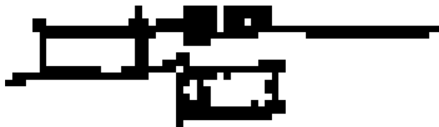
Figure 7.3: Resulting image after applying the Canny and edge detection filters.
