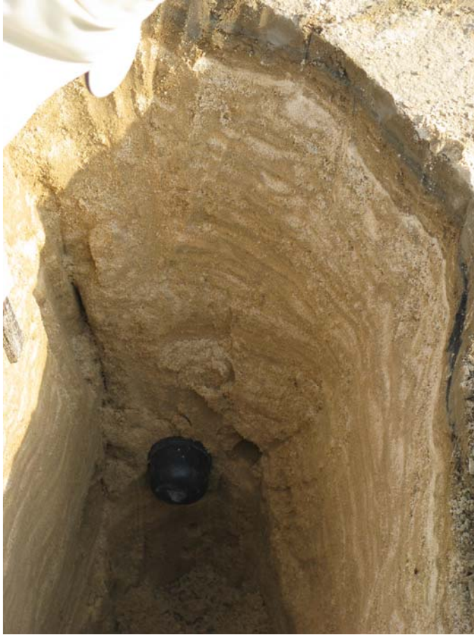
OSL-64 (SUTL2264). 25°41.360N, 49°43.647E. Large sabkha near Hofuf river. 10cm dark sand with black lens over 15cm gypsiferous sand and 53cm of slightly wavy sand. Sample from slightly wavy sand at 53cm.
