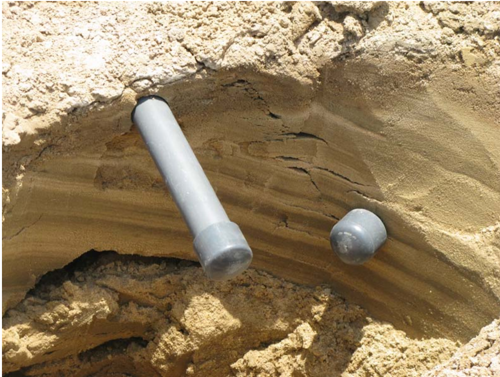
OSL-37 (SUTL2248) and OSL-38 (SUTL2249). 25°46.145N, 50°09.551E. Cross bedded dune sand consisting of an alternation of light and dark laminae (OSL-37), with 10cm of sabkha sediment overlay (OSL-38).
