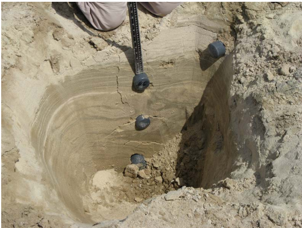
OSL-40 to OSL-43 (SUTL2250-2253). 25°46.685N, 50°08.075E. 8cm sabkha sediment overlaying 13cm ripple sand (OSL-43, top), 12cm low-angle laminated sand (OSL-42), 16cm slumped sand (OSL-41) and 40cm high-angle cross-bedded sand (OSL-40, bottom).
