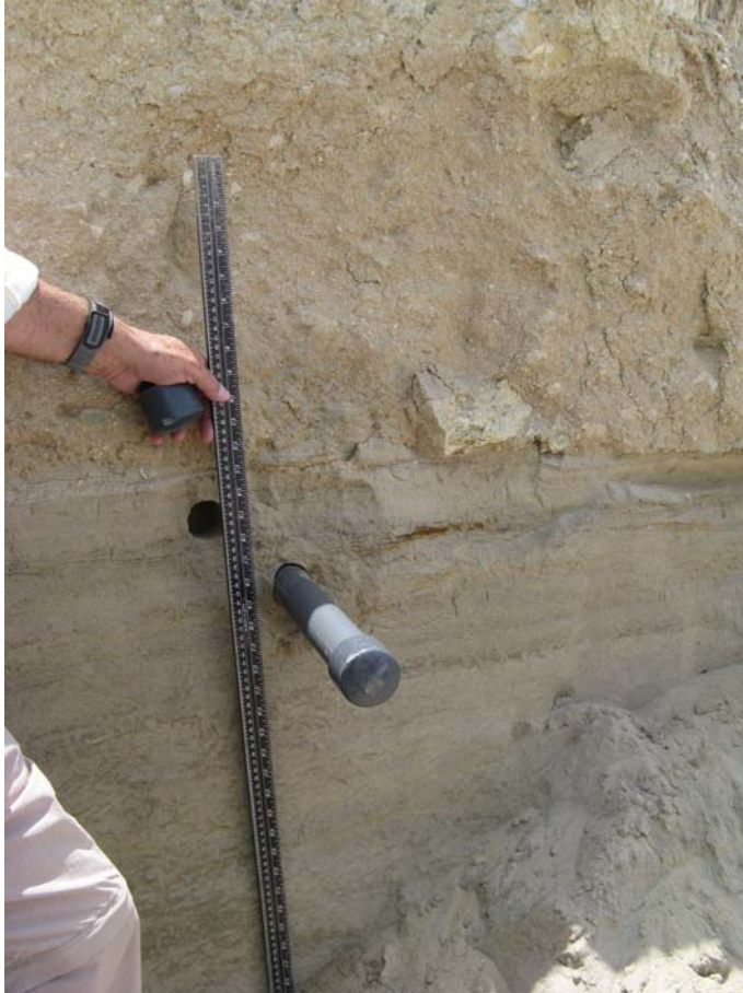
OSL-55 (SUTL2261). 25°48.967N, 50°03.353E. Horizontally laminated sand with bioturbated sand overlay.
