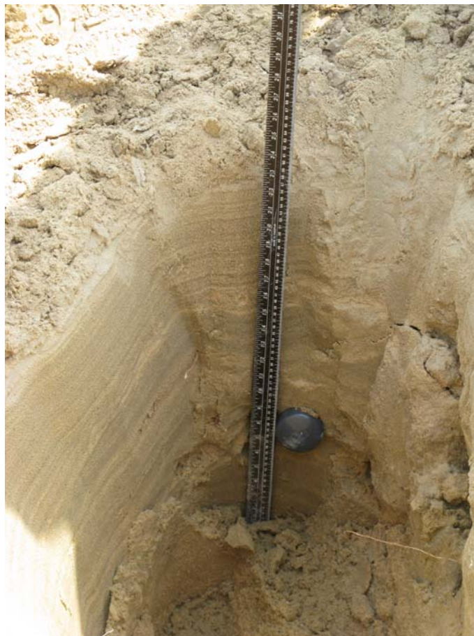
OSL-59 (SUTL2262). 25°44.326N, 49°58.365E. Small sabkha in area of low rolling dunes. Boundary at 20cm depth separating thinner laminated sand, and thicker laminated sand below. Sample from thicker laminated sand at 40cm.
