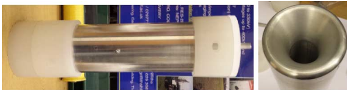
Figure 3. Fully assembled coaxial GIL system. The picture on the right shows the curving radius on the edges of the enclosure wall which reduces end effects.
