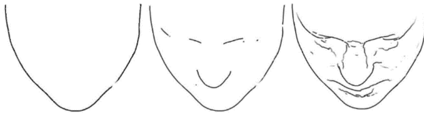
Figure 17: Comparison among contours a) Silhouette contour, b) Silhouette + Occluding contour, and c) Silhouette + Occluding + Suggestive contour of a face model. Image source: (Wuhrer and Shu, 2012).
