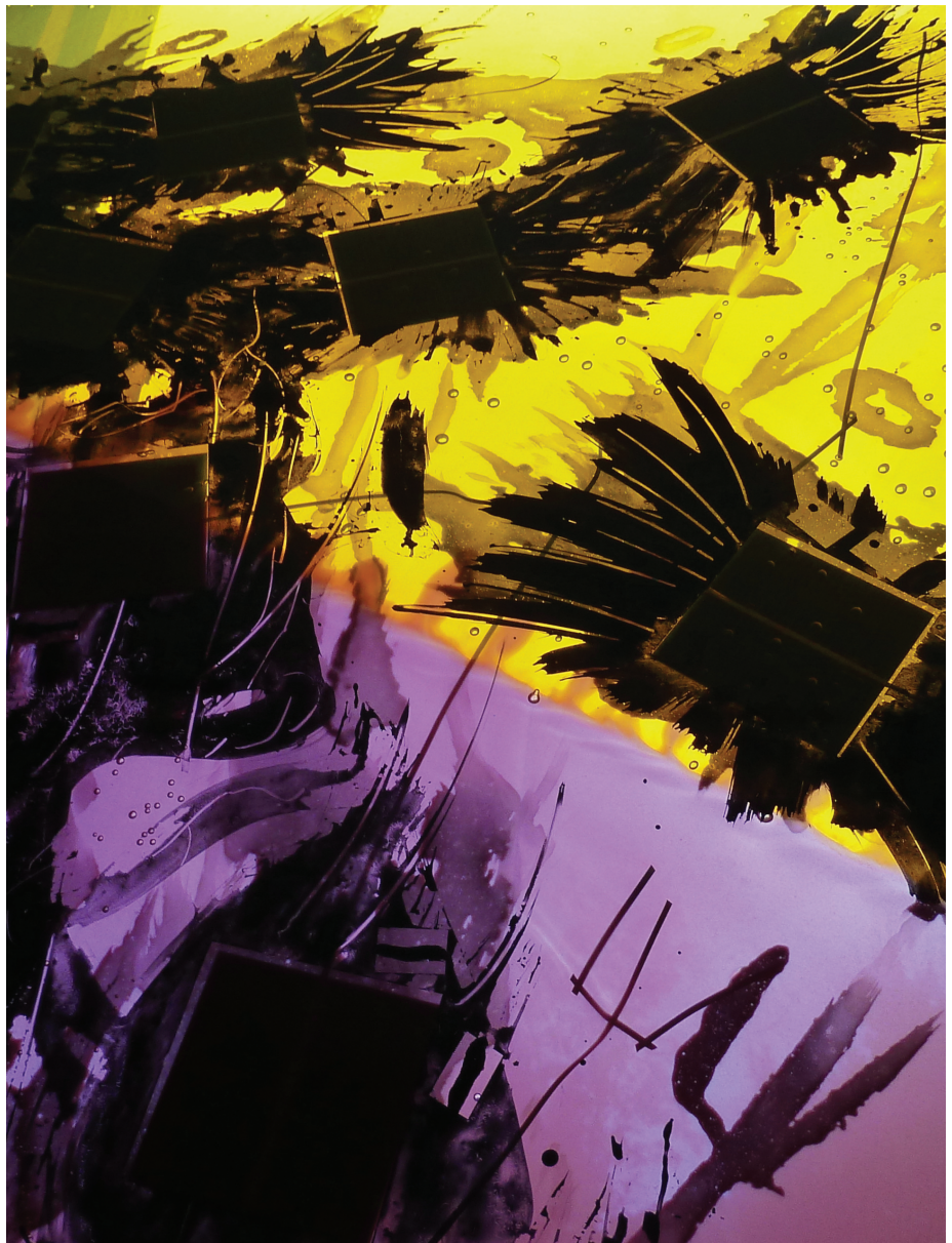
Picture 5 – fluorescent dyes add colour to a painted glass-glass laminate containing solar cells.
