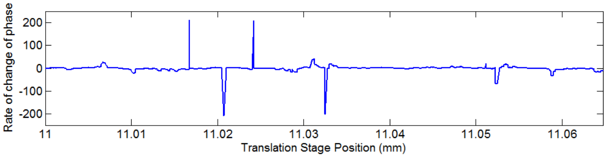
Figure 11.7: The first derivative of the phase, calculated by two-point central difference. Wraparounds can be observed where a large peak or valley occurs.
