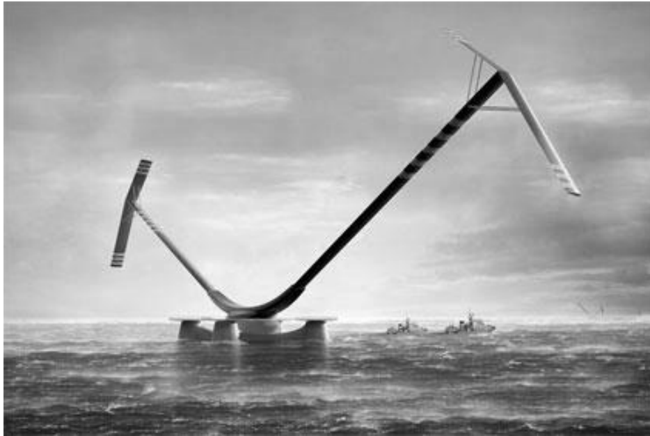
Figure 1.16: V-Shaped VAWT 10MW concept design [25]
