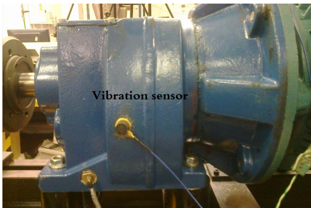
Figure 8 Accelerometer position on gearbox
