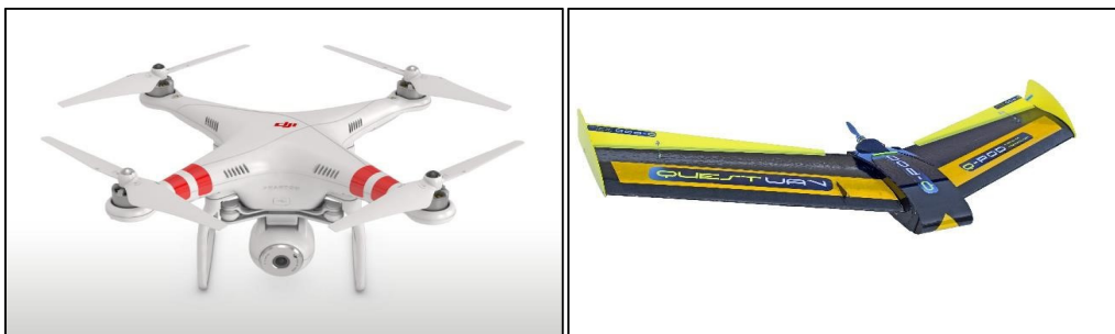
Figure 1. DJI Phantom 2 quadcopter UAV (left) and a Quest Q-Pod fixed-wing UAV (right). UAVs of this size with <20 kg mass and <4 m wingspan are classified as ‘small’ UAVs [24]. (Photographs adapted from [25,26]).
