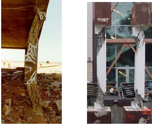
Fig. 14. Field and laboratory-simulated blast tests showing clear shear failure modes in RC columns [Hegemier et al., 2002]
