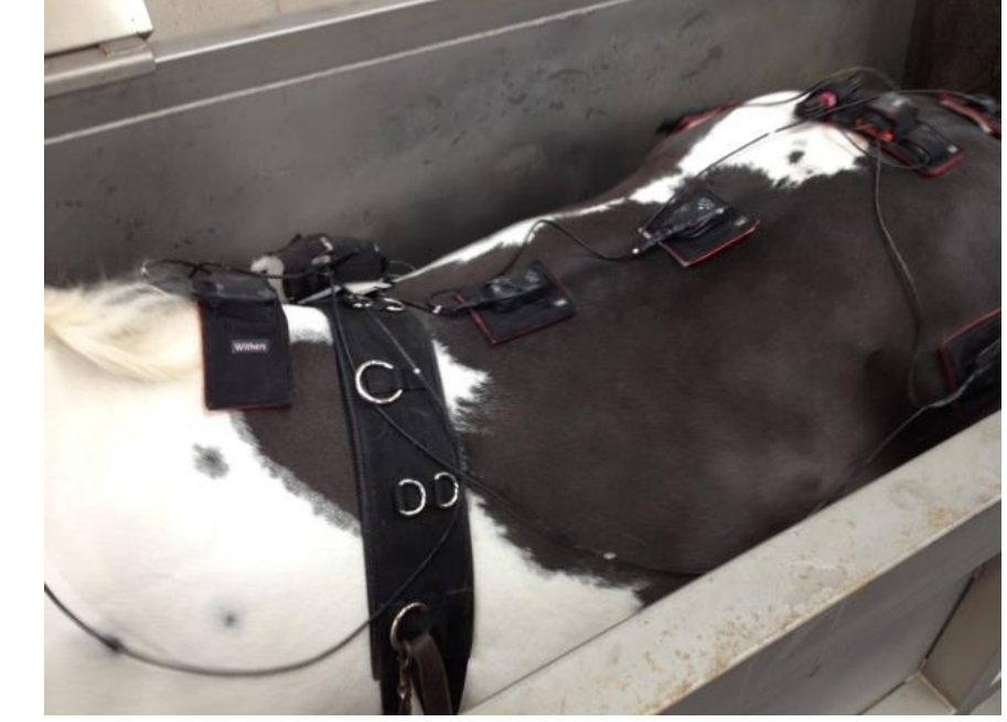
Collecting data on an equine aqua-treadmill using both Qualisys© (a) and Xsens© (b)
