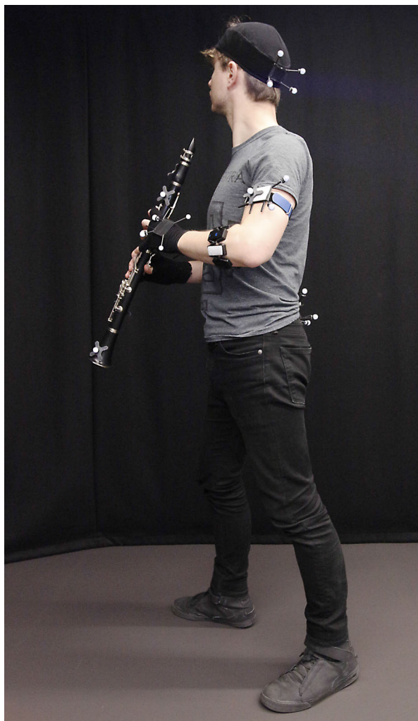
Fig. 9.6 Placement of rigid bodies and Myo armbands for multimodal data recording. The custom rigid bodies are on the back of the head and on the lower back.
