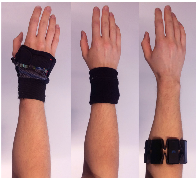
Fig. 8.1 The wearable devices used: fingerless gloves with accelerometers and flex sensors (left), wristband with IMU/MARG sensor (centre), and Myo sensor armband (right).
