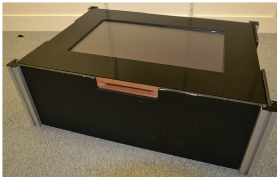
Figure 3.2: Version 1 of the Sandtray touchscreen used in experimental evaluations. A laptop is stored within the wooden housing to run the software, with the touchscreen used as a display.
