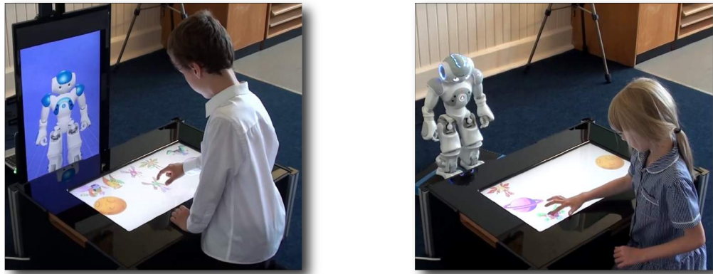
Figure 5.1: Side-by-side images of the virtual ( left ) and real ( right ) robots used for this study: the Aldebaran Nao. The images are stills taken from one of the cameras used for filming. Scaling has been kept consistent between the two images so that size comparisons can be made.
