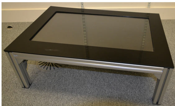
Figure 3.3: Version 2 of the Sandtray touchscreen used in experimental evaluations. This version is much improved, with a sturdier yet smaller construction, larger screen, lighter weight, and built-in computer.
