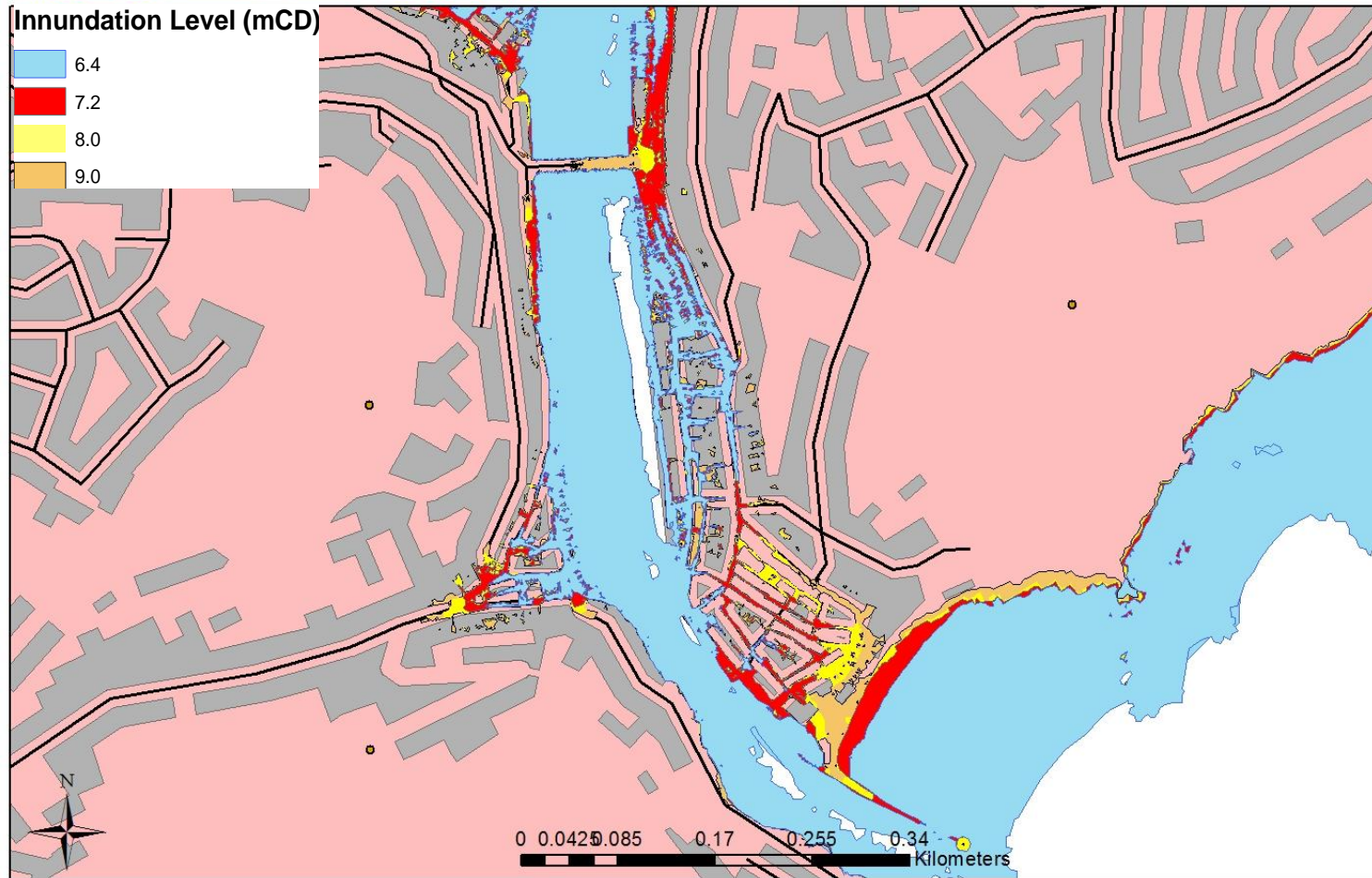
Figure 6.10 LiDAR Digital Elevation Model and Infrastructure Data with Inundation overlay of 6.4, 7.2, 8.0 and 9.0 mCD for Looe, Cornwall.
