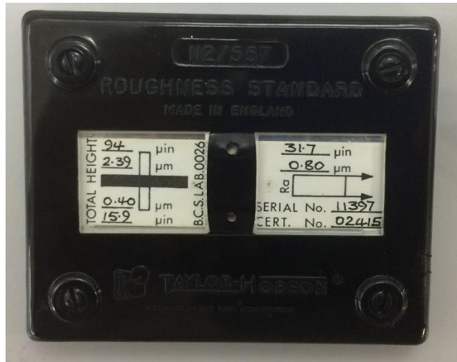
Figure 2-17: Roughness standard used to measure the Ra for 0.8 \mu m
