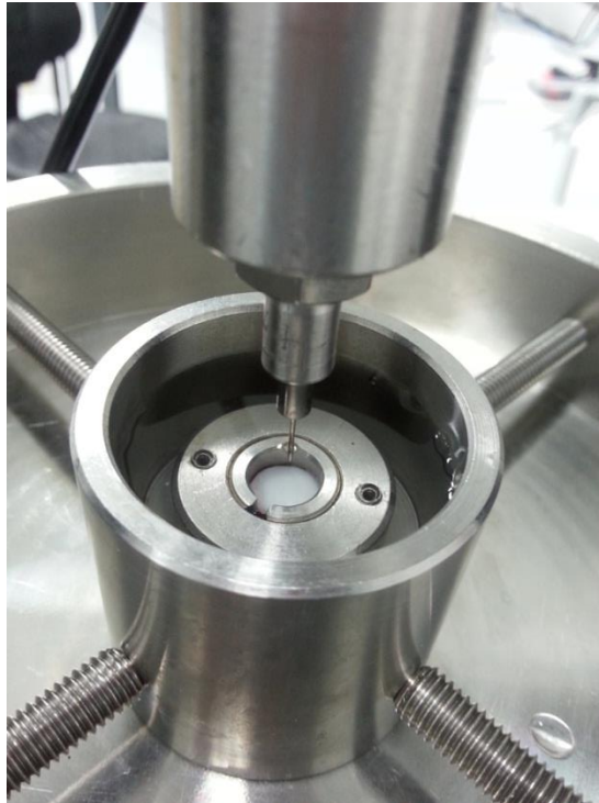
Figure 2-10: The needle attached to the Instron is positioned just above the cartilage
