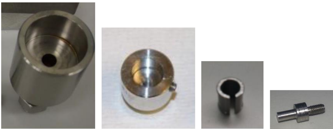
Figure 2-9: From left to right- Stainless steel bath, O ring to fix the collet in place, the collet and flat indenter
