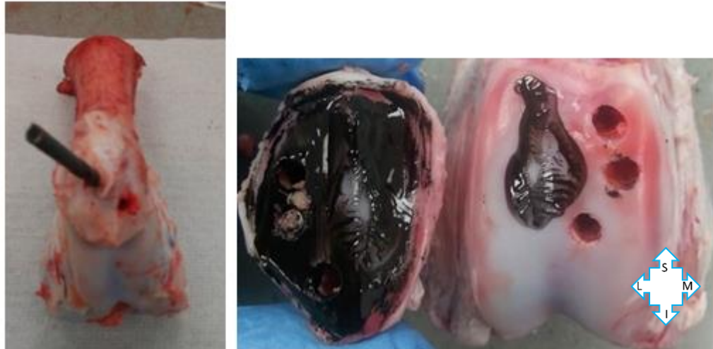
Figure 6-3: Left: Microset applied to the patella cartilage and placed over the femur using the drill holes as guide. Right: The Microset impression from the patella made on the femur representing the contact point.
