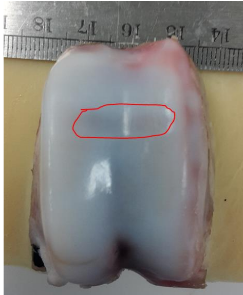
Figure 7-20: The area of deformation caused by the wear study is marked in red
