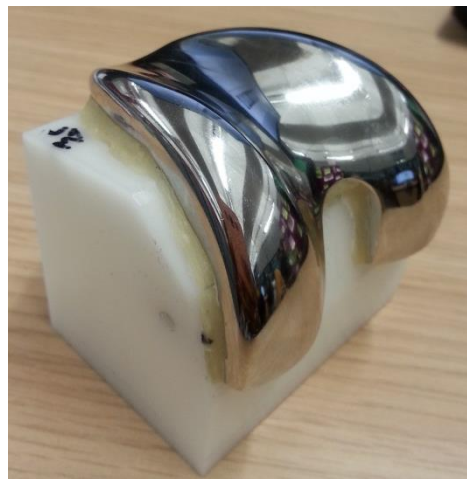
Figure 2-1: Press fit condylar sigma design femoral component used as the positive control
