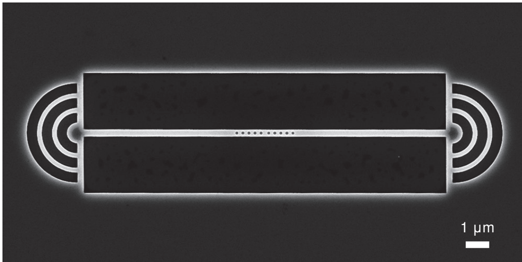
Figure 7.2 – Scanning electron microscope image of a one-dimensional photonic crystal filter within a nanobeam waveguide. Device and image produced by Dr Benjamin Royall.
