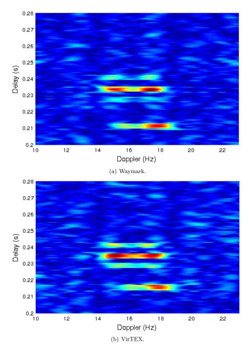
Figure 2.5: CAF for the two propagation models in the winter environment.
