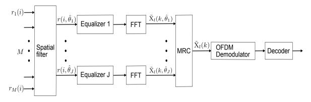
Figure 4.4: Block diagram of the receiver.
