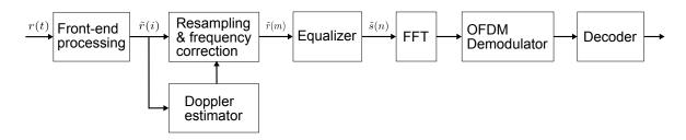
Figure 6.1: Block diagram of the receiver of guard-free OFDM signal.
