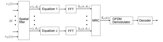
Figure 6.6: Block diagram of the receiver (for convenience, we show Figure 4.4 again).
