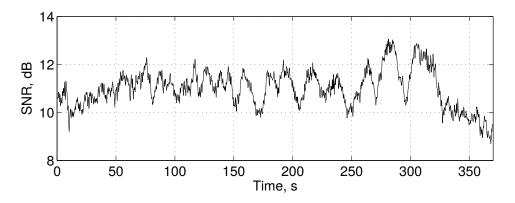
Figure 3.12: Time-varying SNR in the F1-10 sea trial.
