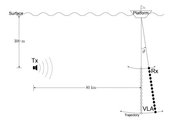
Figure 5.4: Simulation scenario with periodic oscillating receive VLA. Tx is the transmitter, and Rx is the receiver.
