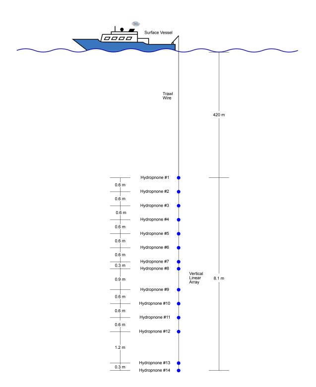
Figure 4.1: Vertical Linear Array of 14 hydrophones deployment in the sea trials.
