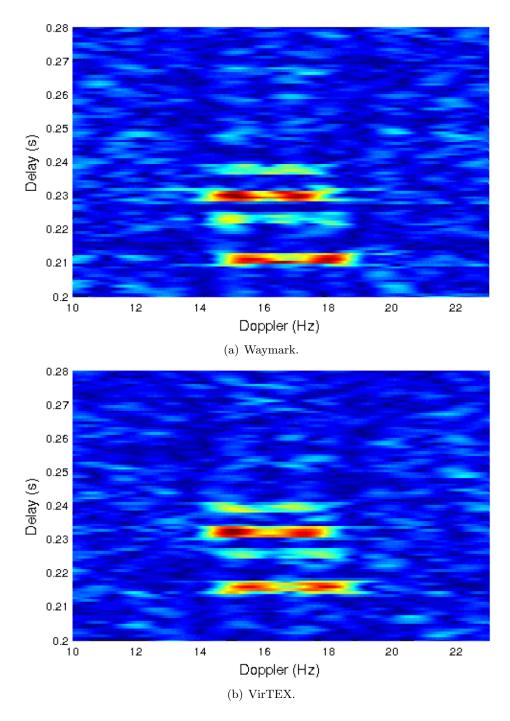
Figure 2.4: CAF for the two propagation models in the summer environment.
