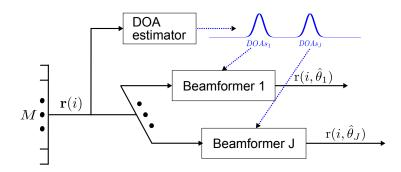
Figure 5.3: Block diagram of the spatial filter with J outputs based on J space clusters.
