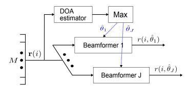
Figure 4.7: Block diagram of the SF with J outputs based on maxima of the spatial signal power.
