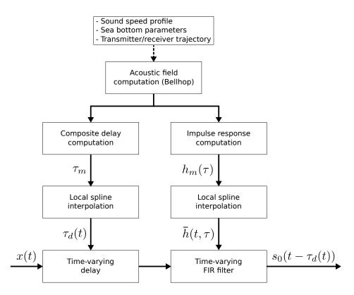
Figure 3.2: A block diagram of the Waymark underwater acoustic simulator; adapted to this chapter.
