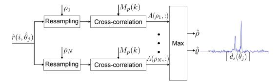
Figure 4.9: Block diagram of the Doppler estimator.
