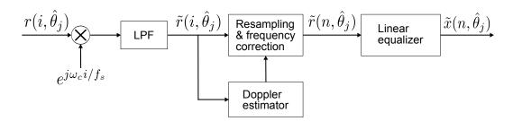
Figure 4.8: Block diagram of the equalizer.
