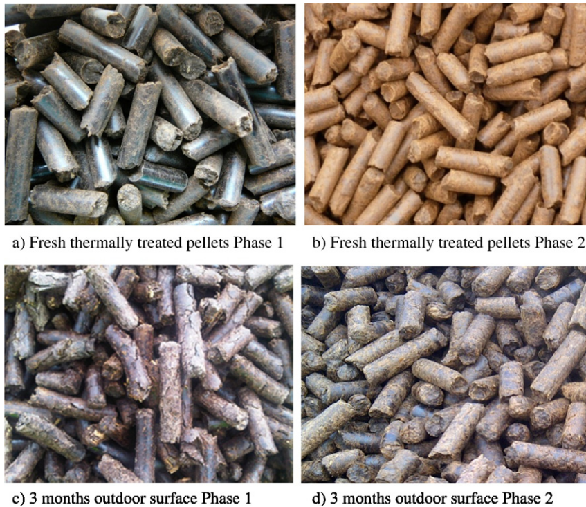
Fig. 3. Fresh and stored pellets after 3 months in storage from Phase 1 (a + c) and Phase 2 (b + d) outdoor steam exploded pellet piles, where fresh is used to denote pellets at the start of the storage period.
