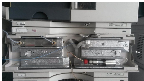
Figure 7: RD2 held in place within the thermostatted Agilent 1100 series column department.
