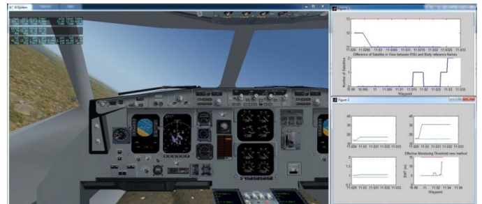
Fig. 30. Real-time ARAIM computation integrated into the X-Plane software
