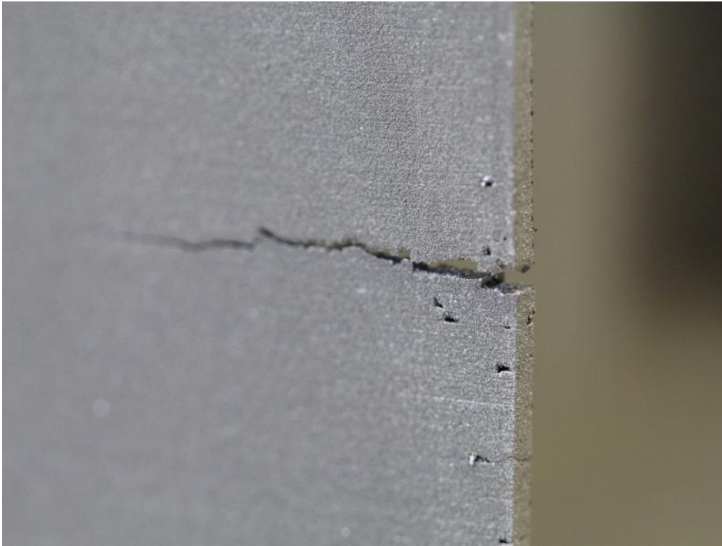
Figure 1 - Failure during manufacturing of a Ti-6Al-4V component caused by the build-up of residual stress.
