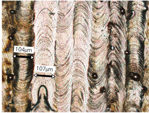
Figure 7 – a) Single layer laser scan on a base plate using Ti-6Al-4V of adjacent tracks and b) diagram illustrating the calculated overlap of adjacent scan tracks for the simulation.
