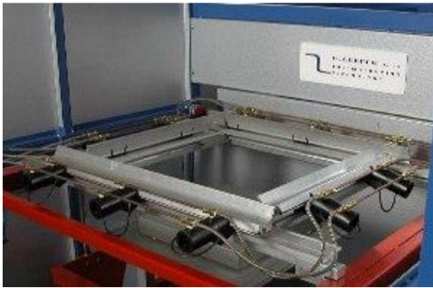
Figure 2. Example of a thermoforming clamp frame for the use in vacuum forming [11].
