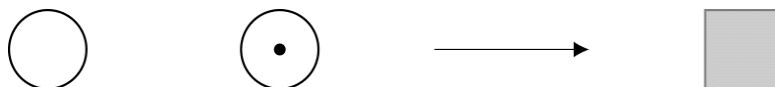
Figure 1: Components of a Petri-Net. From left to right: unmarked place; marked place; arc; transition.
