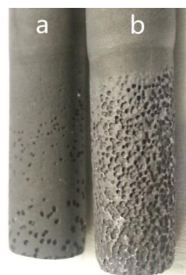
Fig.5 Anodes electrolysed with tube and without tube. (a. off side with hole, b. off side without hole)
