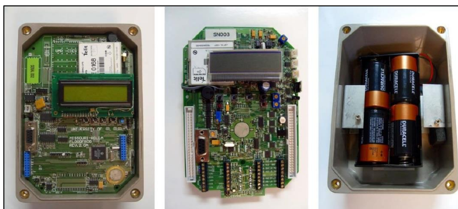
Figure 2-9 SmartBrick revision 2.0 (left), 2.1 (center), and the IP68 SmartBrick enclosure (right) (Harms et al., 2009a).
