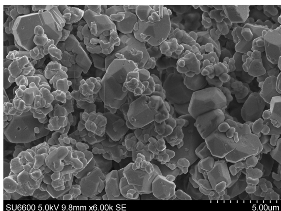
Figure 4. SEM images of spray-dried CBZ IV.
