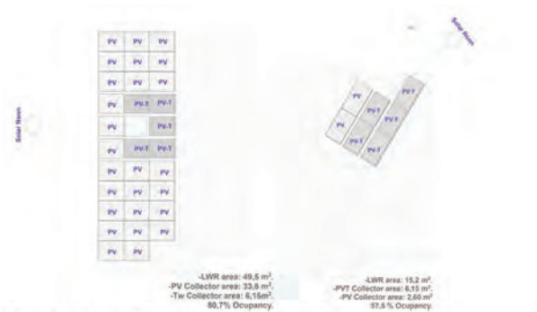
Figure 5 (a) Capacity of PV and PVT collectors in Models A y B.
