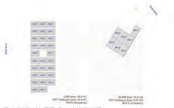
Figure 6(a) Capacity of PVT collectors in Models A y B.
