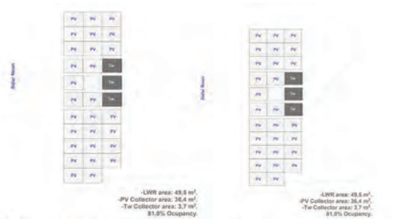
Figure 4 (a) Capacity of PV and Tw collectors in Models A y B.
