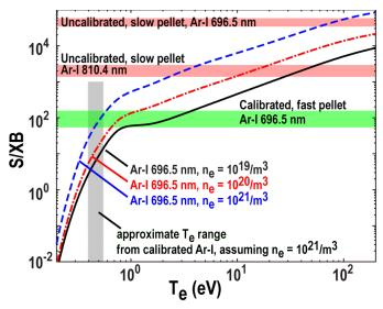
Figure 7. Curves of theoretical photon efficiency S/XB for Ar-I 696.5 nm vs  $T_e$  and range of S/XB seen in fast pellet experiments. Absolute (scale) for uncalibrated data is arbitrary; data is shown to illustrate low shot-shot scatter in *S/XB*.
