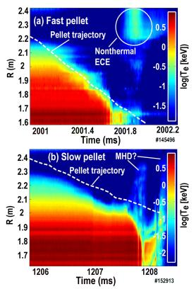
Figure 4. Examples of ECE contours vs major radius and time and pellet trajectories for (a) fast pellet and (b) slow pellet.
