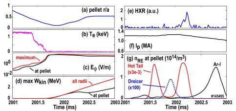
Figure 9. Time traces for fast pellet of (a) pellet location, (b) central electron temperature, (c) Toroidal electric field at pellet (and maximum across whole profile), (d) maximum RE kinetic energy at pellet (and across whole profile), (e) HXR signals, (f) toroidal plasma current, and (e) RE density at pellet location.
