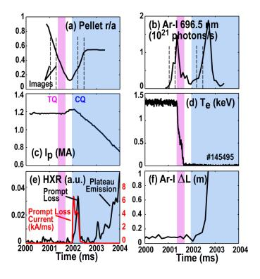
Figure 2. Overview of time traces and sample Ar-I pellet images showing (a) pellet location (in terms of normalized plasma minor radius  $\rho = r/a$ ), (b) Ar-I brightness, (c) plasma current, (d) plasma central electron temperature, (e) hard x-ray emission, and (f) ablation plume length (from Ar-I emission) vs time. HXR vertical scale in Fig. 2(e) is same as for Fig. 1(e).
