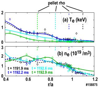
Figure 5. Burst mode Thomson profiles of (a) electron temperature and (b) electron density during slow pellet trajectory showing little density perturbation far from pellet toroidally.
