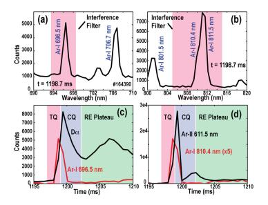
Figure 6. Survey spectrometer data of slow Ar pellet emission showing: (a) a sample spectrum in the vicinity of Ar-I 696.5 nm, (b) a sample spectrum in the vicinity of Ar-I 810.4 nm, (c) time traces of Ar-I 696.5 nm and D $\alpha$  656.2 nm, and (d) time traces of Ar-I 810.4 nm and Ar-II 611.5 nm.
