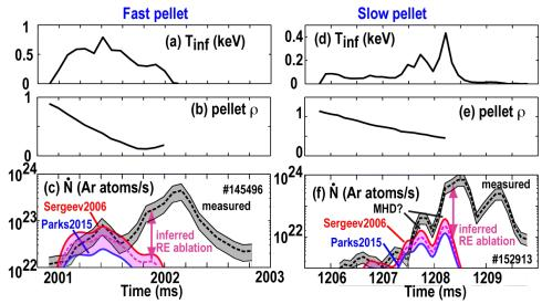
Figure 8. Comparison between measured and predicted Ar ablation rate for fast pellet (left side) and slow pellet (right side). Data shows time traces of (from top to bottom)  $T_{\infty}$  ( $T_{\rm e}$  toroidally far from pellet), pellet position (normalized minor radius), and measured and modeled ablation rate.
