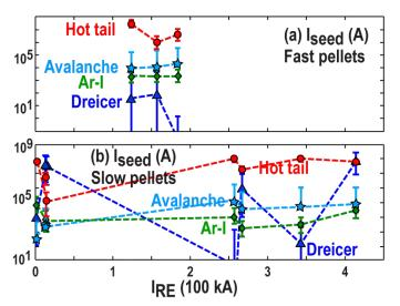
Figure 10. RE seed current at end of TQ estimated for (a) fast pellets and (b) slow pellets as a function of initial RE plateau current.
