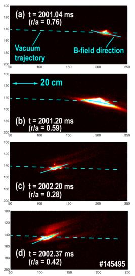
Figure 3. Sample Ar-I 696.5 nm images at times corresponding to vertical dashed lines in Fig. 2(a,b).
