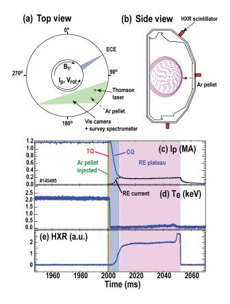
Figure 1. Schematic of experiment showing (a) top view and (b) side view. Ar pellet trajectory and main diagnostics used here are shown. Also shown are time traces giving overview of typical experiment conditions showing (c) plasma current, (d) thermal electron temperature, and (e) hard x-ray emission. Vertical color bands serve only to illustrate different phases of disruption.
