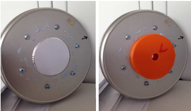
Fig. 2. Ultrasound Loudspeaker (left) as the air-coupled transducer used in the measurements. Assembly transducer-cylindrical structure (right) as one of the emitters.
