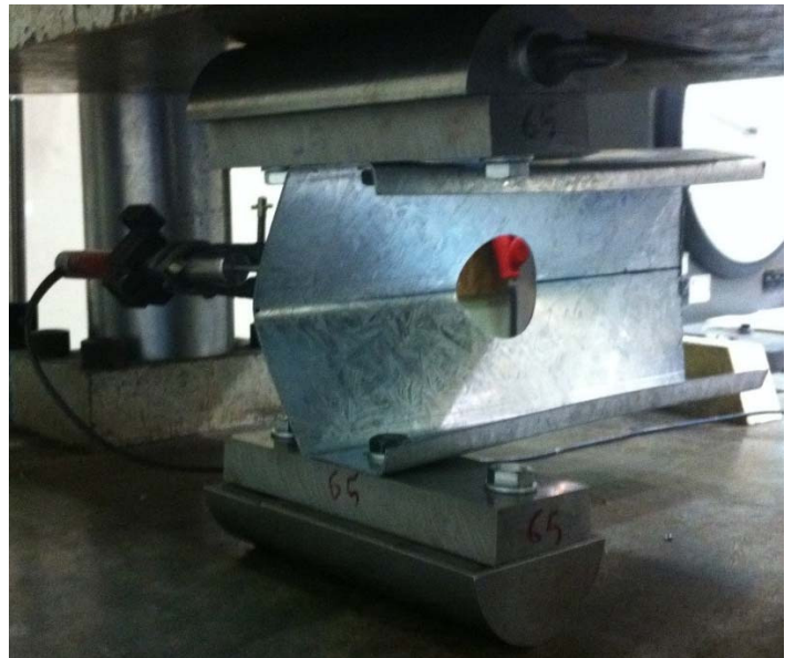
(b) Offset circular web opening
