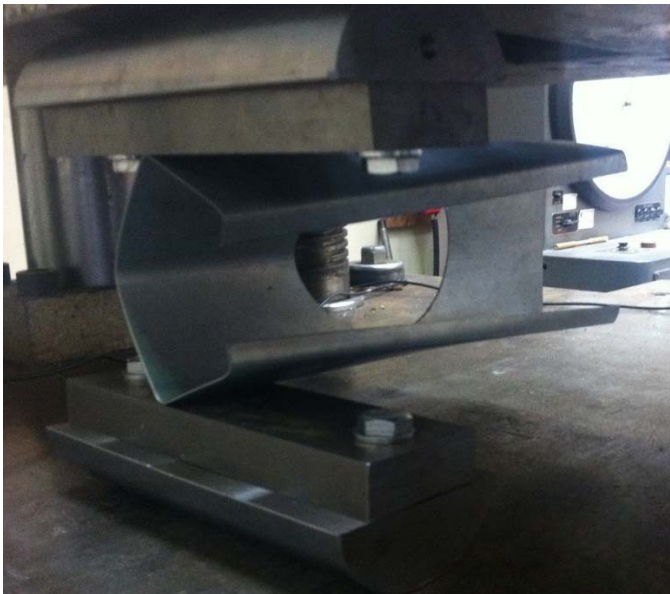
(b) Offset circular web opening
