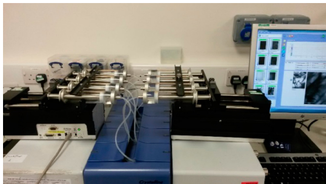
Figure 2. Technobis Crystalline and syringe pumps for solubility determination using the solvent addition method.
