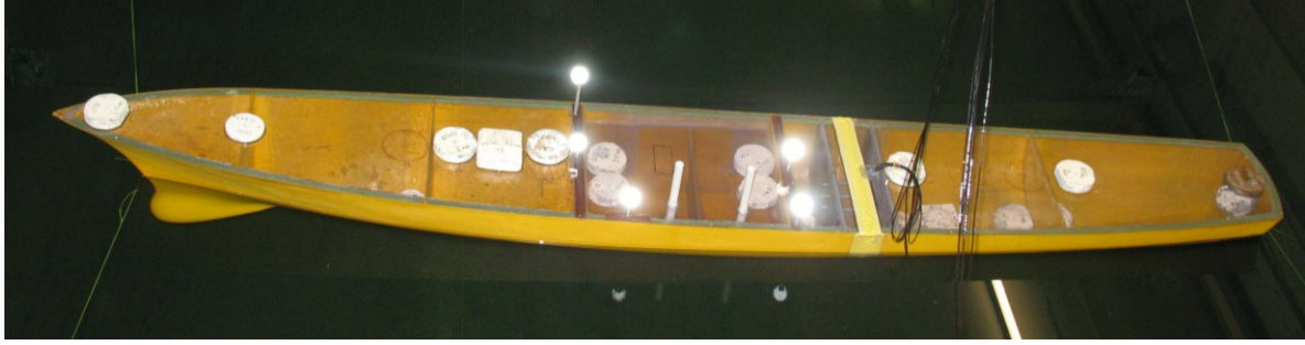
Figure 1. DTMB 5415 model, positions of bulkheads and load cell
