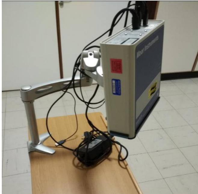
Fig. 6 2. The MoorFLPI full-field perfusion imager for recording the blood perfusion in digits.
