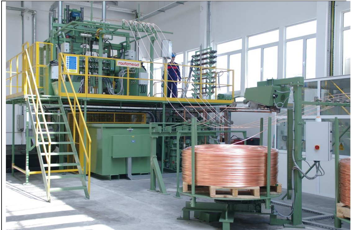
Figure 2-7: Vertical continuous casting factory ( http://www.rautomead.co.uk )
