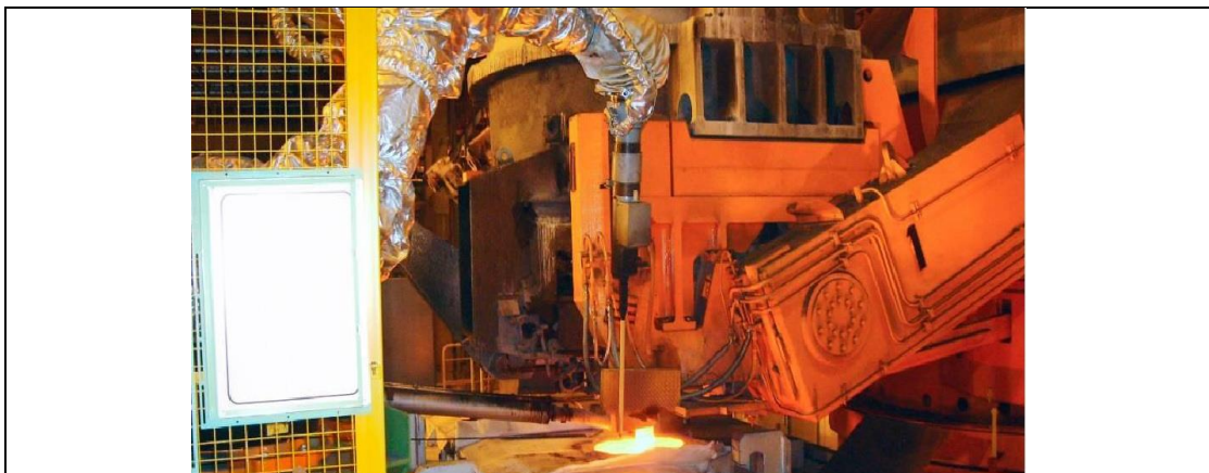
Figure 2-3: LiquiRob during temperature measurement at POSCO Gwangyang for temperature measurement in continuous casting of steel slab (Juergen Meisel, 2014)
