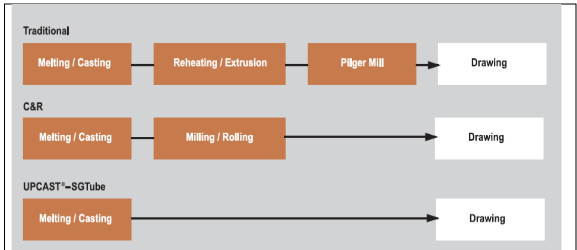
Figure 5-1 (c): Schematic of various DHP copper tubes manufacturing process (UPCAST, 2013)
