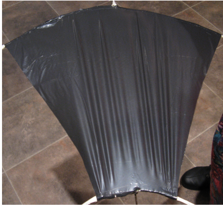
Figure 6.1: Wrinkle configuration exhibited in a stretched annular segment of a plastic bag. Tensile stress is applied radially outwards along the inner and outer edges. Wrinkles form at the inner edge of the annular segment, and different penetration depths can be observed for individual wrinkles i.e. some wrinkles extend further into the domain than others.
