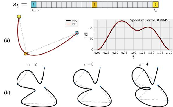
Figure 5: Interpolation with MPC. **a**, comparison of MPC (black) with a closed form solution of a minimum jerk trajectory with 1 via-point (red). On top, a color coded schematic of the corresponding state vector. **b**, examples of interpolating trajectories of increasing order (2, 3, 4).
