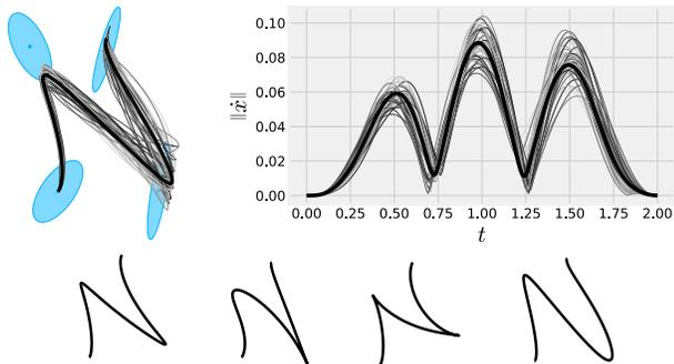
Figure 4: Stochastic sampling of the trajectory distribution for a letter “N”. **Top-left:** the mean trajectory (black), random samples from the trajectory distribution (gray) and the corresponding Gaussians. **Top-right:** The corresponding speed profiles. **Bottom:** Selected random samples from the trajectory distribution.
