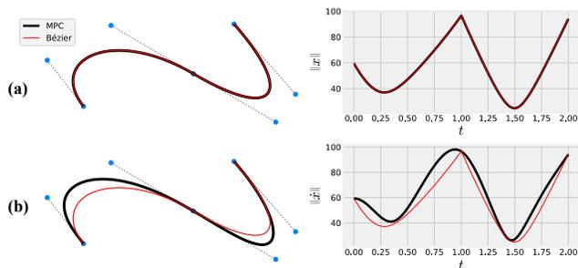
Figure 6: Approximating Bézier curves with a sparse reference and states augmented with velocity. **a**, 2nd order system, which results in an identical curve and speed profile (as shown in [14]). **b**, the same states with a 3rd order system. This produces a slightly different curve with a higher degree of continuity.
