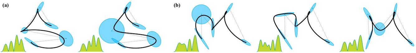
Figure 3: **(a)**, smoothing effect of increasing the variance of a Gaussian. **(b)**, manipulating the trajectory evolution with full covariances. Below each trajectory, its corresponding speed profile.
